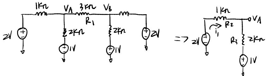
because of Symmetry,  $V_A = V_B$ , and there is no current flowing through  $R_1$ .
